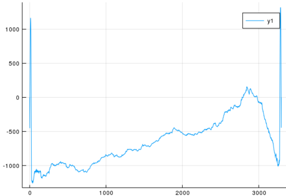
FIGURE 4.1: The result of doing BIC on an audiotrack. Where the x-axis shows the frame number and the y-axis shows the score from the BIC in that frame
