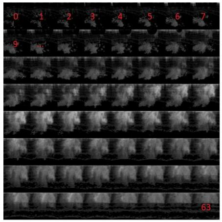
*Figure 36: Example of a texture atlas containing 64 smaller images. Some of the images has a number showing their index*
