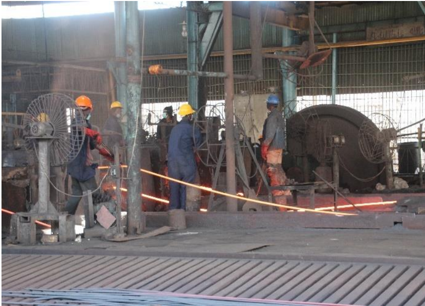
Figure 8: steel manufacturing using a rolling mill machine: Droning noise from multiple operating six-strand rolling machines, flywheels, electric fans, motors, conveyor rails, frequent collision of metal rods in motion and hammering.
