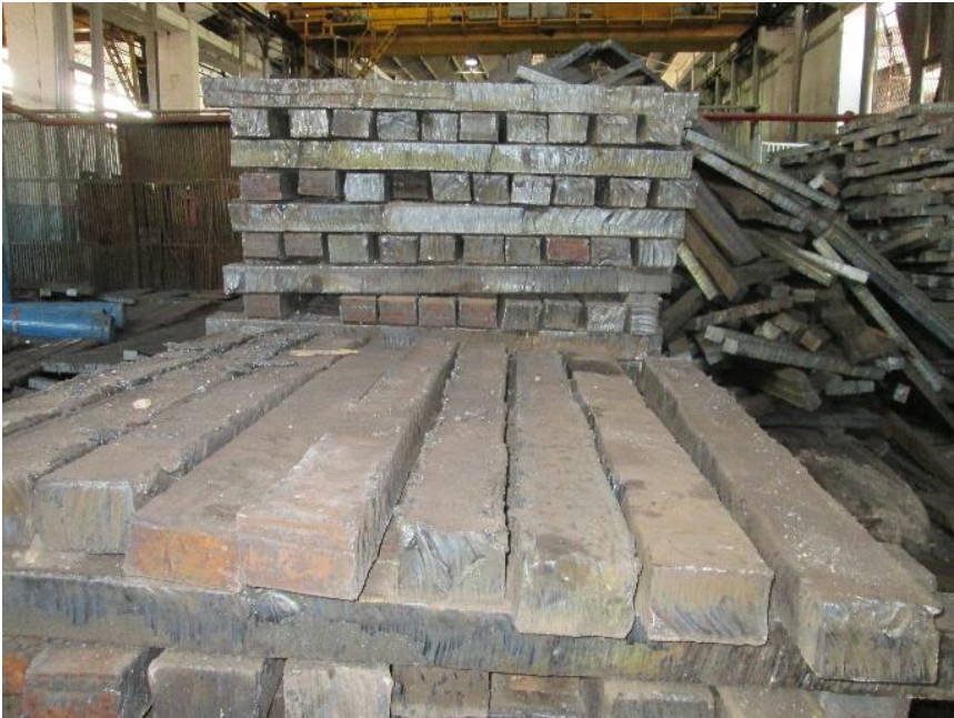
Figure 4: steel billets made from domestic scraps: Two different billet weights (100-120kgs vs 20-30kgs) were used in the rebar production process. The large billet weight was related to higher noise levels than the smaller billet weight.
