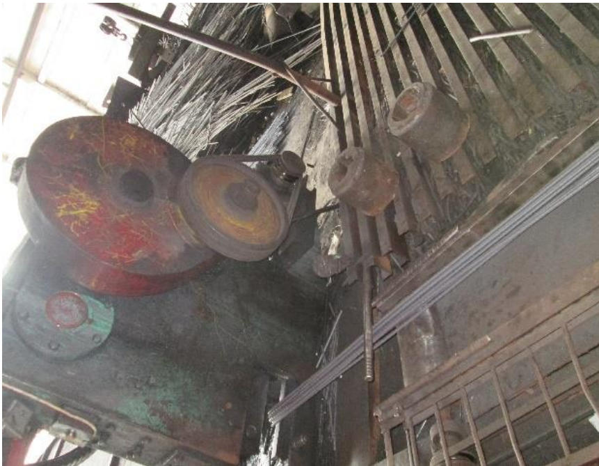
Figure 9: steel cutting into 6-metre length: large cutting machines produce higher noise levels than the smaller cutting machines
