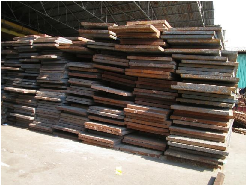
Figure 5: imported steel billet sheets, normally cut into larger billet weight for rebar production
