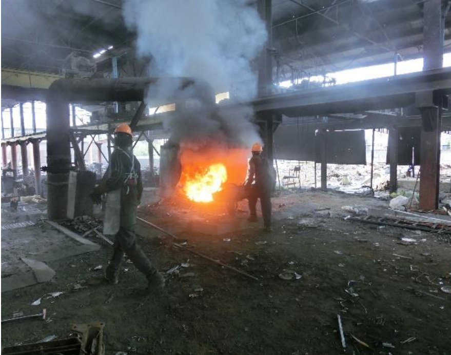
Figure 6: feeding a furnace oven with metal scraps: droning noise from operating furnace, noise from collision of metal scraps during furnace feeding, loading handcart and siren. Noise from explosive materials accidentally fed into the furnace.
