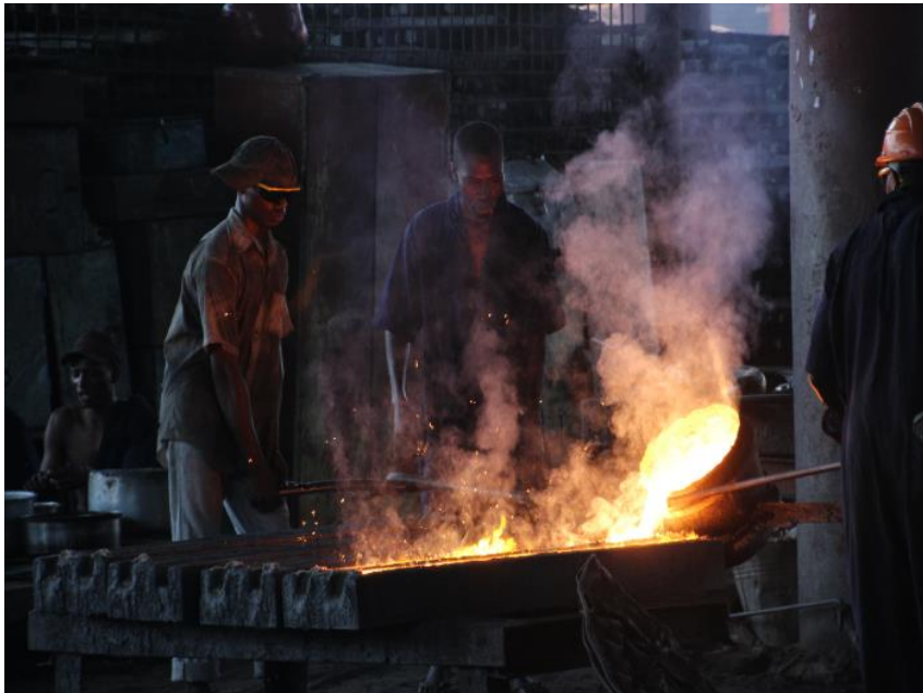
Figure 7: Pouring molten steel into moulds
