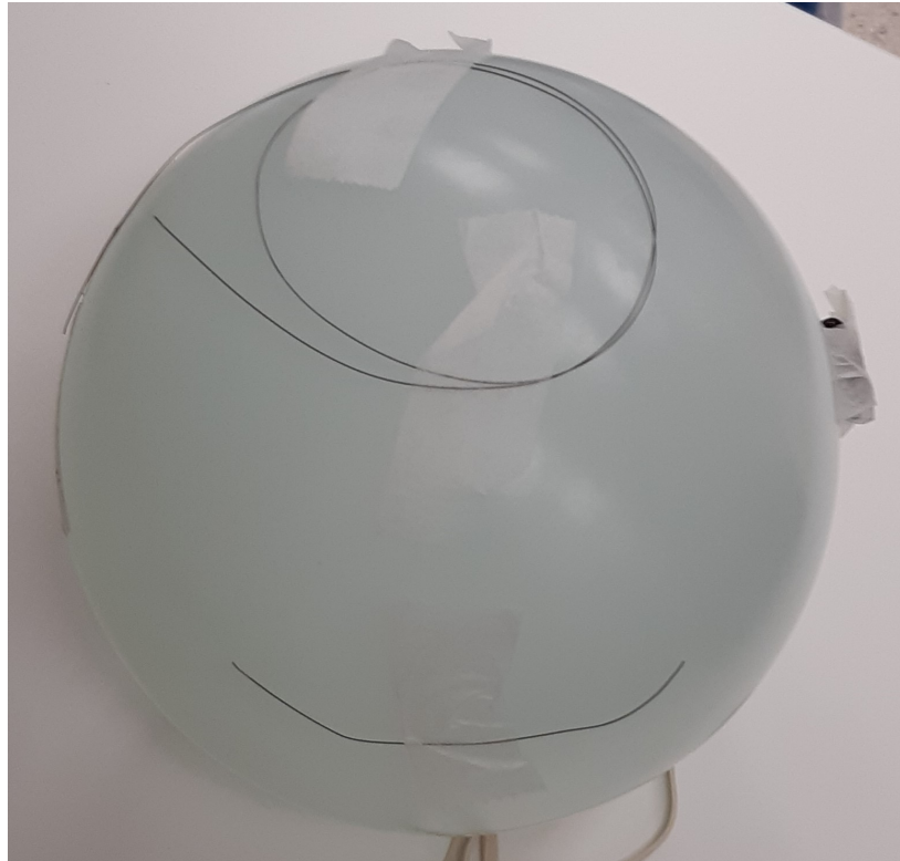
FIGURE 4.14: MRI visibility testing: material placement on phantom - back
