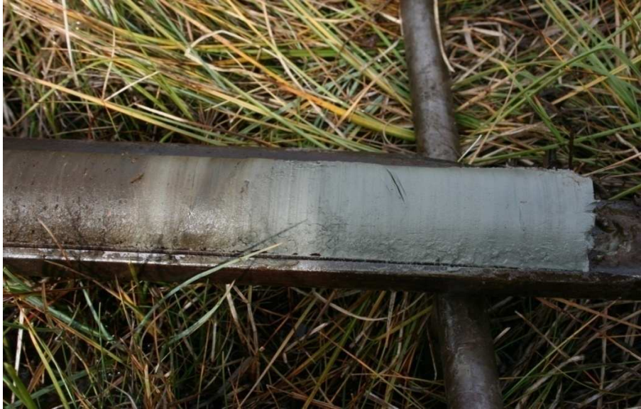
Figure 3.1: The figure shows the lowermost minerogenic sequence of a test core obtained with a 54 mm Russian corer at the Lervahå mire, September 2008. Photo: Vanja Haugland
