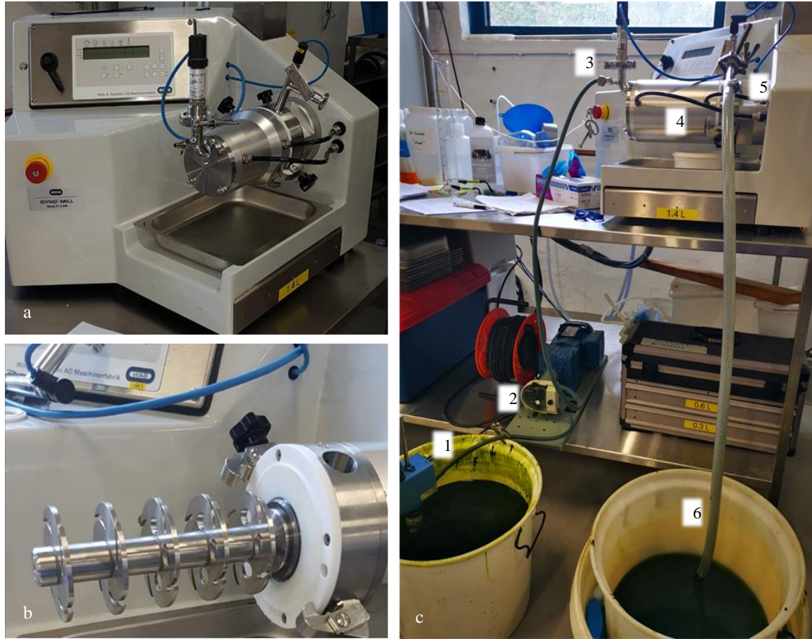
Figure 2: Dyno-Mill Multi Lab (WAB). (Photo: Kokkali) a) The agitator bead mill with with 0.6 l grinding container and digital display. b) The agitator discs mounted on the agitator shaft c) 1: unprocessed biomass mixing, 2: pump which “feeds” the mill, 3: product inlet, 4: 0.6 l grinding container (chamber), 5: product outlet, 6: disrupted biomass collected on cooled.
