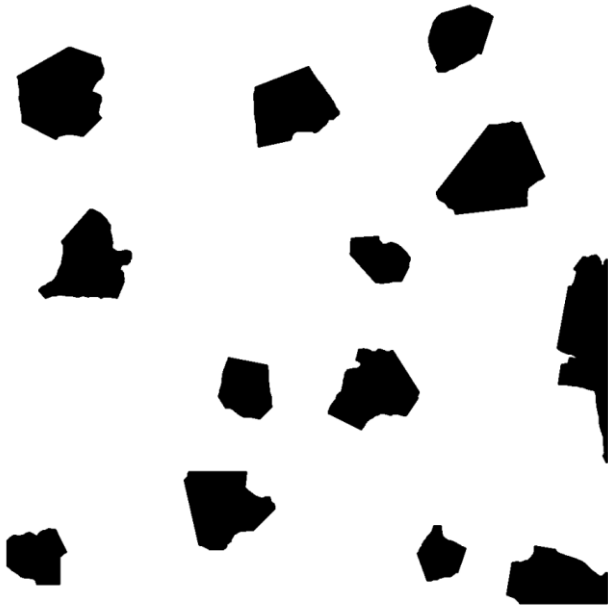
Figure 46: Image showing the threshold of the previews image using the described threshold function. These shapes were then converted to contours and then polygons, so it is possible to find the intersection between them and the lines.
