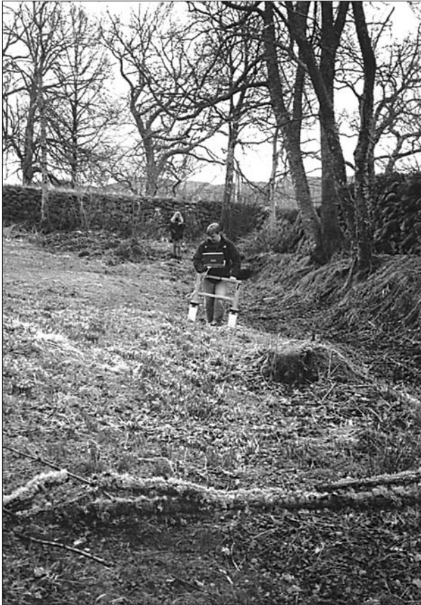
12. - Georadar used from the south-eastern part of the garden crossing the large "Dam" (see fig. 8 and 13, photo DM).
