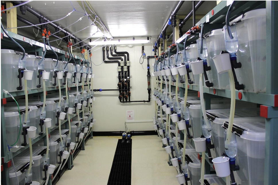
Figure 8: Single fish tank arrays. Wet-lab facility at the SLRC used in salmon louse experiments. Each tank holds one salmon with salmon lice. Photo: Lars Are Hamre.
