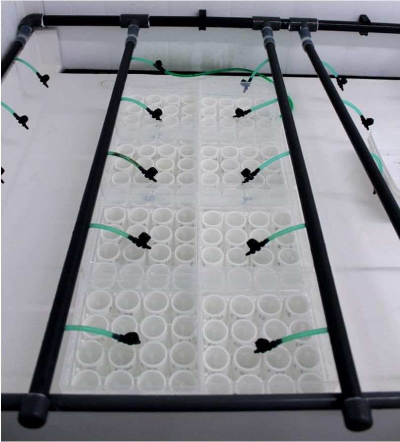
Figure 7: Salmon louse incubators. Incubators with individual hatching wells used to keep and observe egg strings and the developing salmon louse larvae. A continuous supply of sea water is obtained through the green tubes. Photo: Lars Are Hamre.
