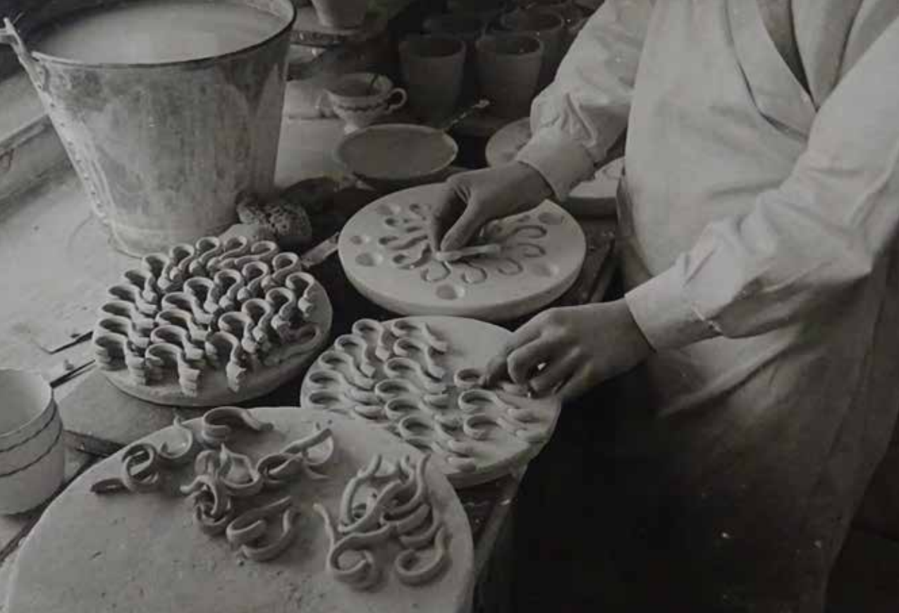
Fig. 3. 'Handles for Cups and Jugs are cast with the same meticulous care.' Mintons Ltd, Stoke-on-Trent, 15 March 1946
