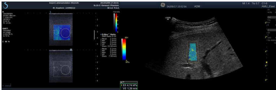
Figure 4. An illustration of commercially available SWSI methods, demonstrated in vitro on a tissue-mimicking inclusion phantom (Model 049 Elasticity QA Phantom, Computerized Imaging Reference Systems Company [CIRS], Norfolk, VA, USA), with 2D-SWE, SSI (Aixplorer, Aix-en-Provence, France) to the left, and in vivo on a healthy subject with 2D-SWE, LOGIQ E9 (GE Healthcare, Milwaukee, Wisconsin, USA) to the right. Images: A. Mulabecirovic
