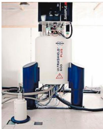
Figure 32. MR spectrometer MR Spectrometer for high-throughput analysis of tissue and biofluids. Photo Geir Mogen
