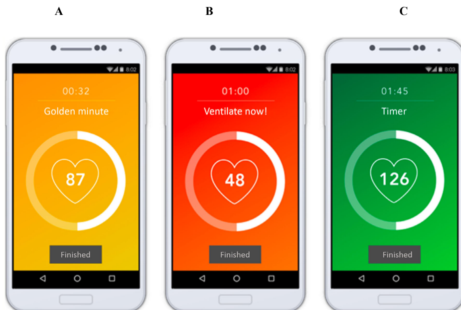
Figure 12. (A, B and C) The NeoTapLS as displayed on the phone screen. Heart rate is registered by tapping at least 3 times on the screen. (A) Heart rate at 32 seconds <100 (yellow screen), prepare for ventilation. (B) Heart rate at one minute <60 (red screen), ventilate now! (C) Heart rate at one minute 45 seconds >100 (green screen), ventilation is satisfactory.
