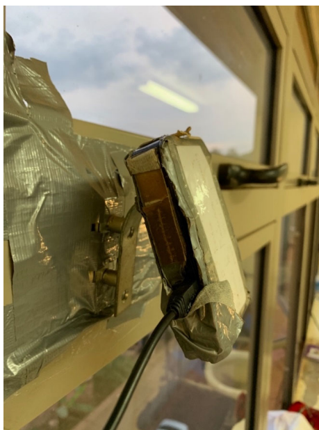
Figure 11. Camera attached on magnetic mount. Casing concealed under duct tape to absorb shocks and discourage theft. (Photo: Nicolas Pejovic)
