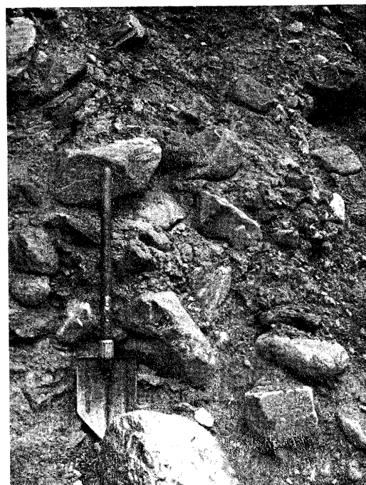
Fig. 12. The uppermost stoney till, B, which is interpreted as an ablation till. The material is coarse and the content of far-transported, often rounded particles is higher than in the basal tills.
