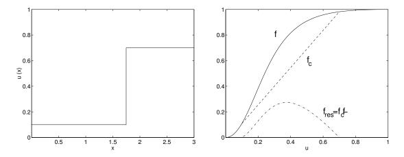
FIGURE 1. (Left) A single shock solution from a convection step. (Right) The corresponding residual flux function; flux function f (solid), convex envelope  $f_c$ , i.e., local linearisation (dash), and residual flux  $f_{res}$  (dash-dot).
