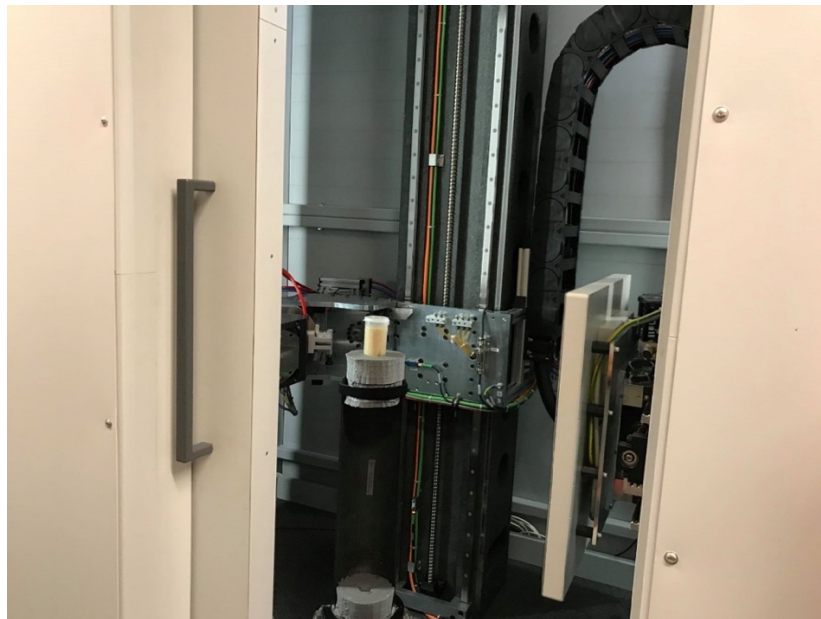
Figure 3.12: A core plug placed inside the CT-scanner at the Department of Earth Science.
