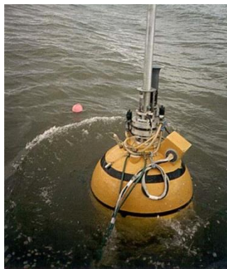
Figure 5. Photography of Norwegian power buoy [20]
