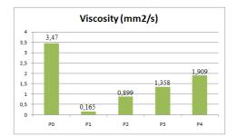
Figure 3. Viscosity of the Sargassum sp. biodiesel.
