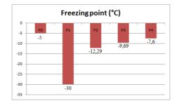
Figure 2. Freezing point of the Sargassum sp. biodiesel.
