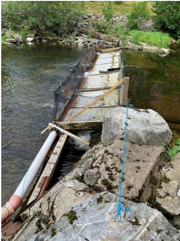
FIGURE 6. Wolf trap set-up in the river Dale
