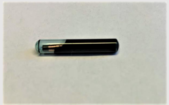
FIGURE 1. 12 mm HDX PIT-tag (Biomark)
