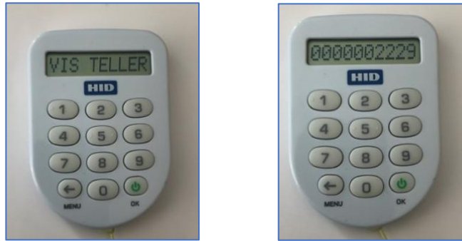
Figure 8: A picture of the token model HID Pocket token provided by Nordea and the inbuilt counter function. It is possible to see that this particular token has in total generated 2229 passwords.
