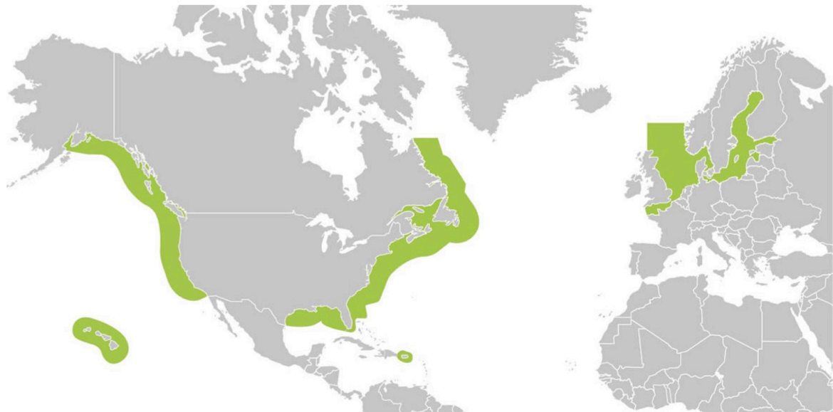
Figure 2: The green areas on the map marks the Emission Controlled Areas (ECAs) set by the IMO. These areas are classified as especially vulnerable areas for maritime activity by the IMO [4]
