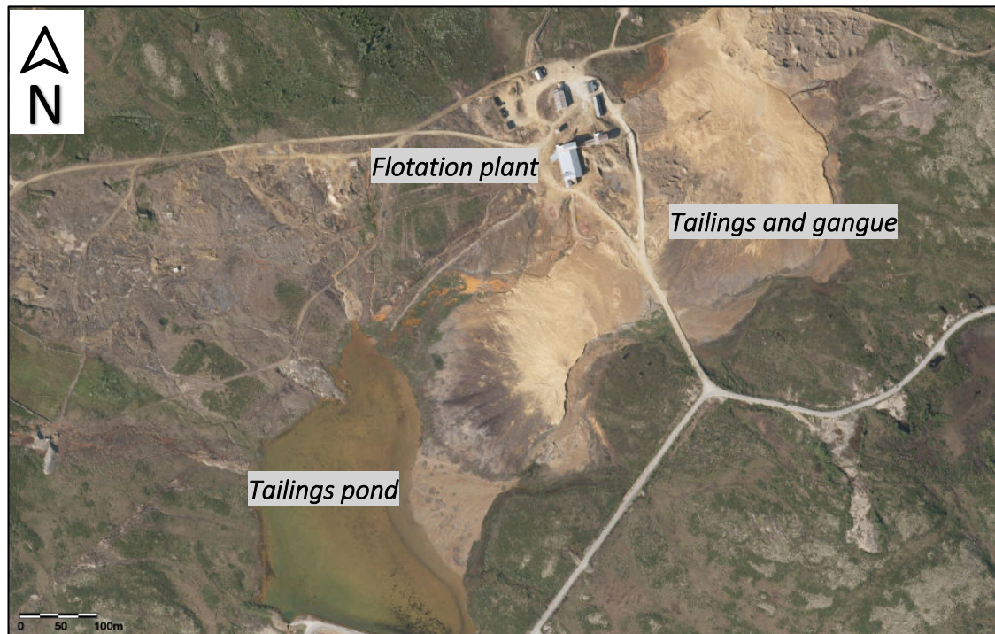
Figure 3.2: Lower Storwartz where the flotation plant was built. The tailings pond, Slamdammen, used for under water disposal of tailings. Large exposed waste piles of tailings and gangue also clearly visible in the area. Made with Norge i bilder (2020).
