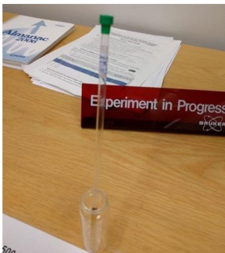
Figure 3-6 NMR samples for AV500 and AV600
