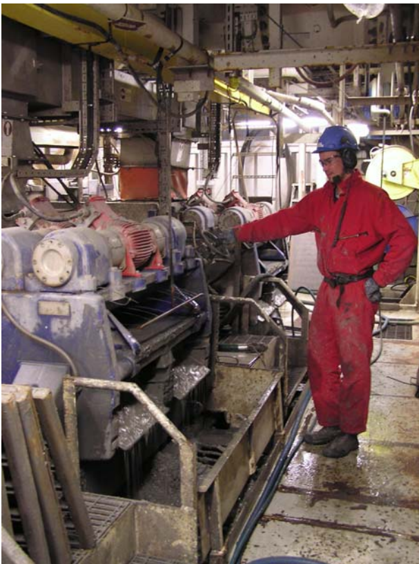
Figure 8. Operator surveying open shale shakers at Oseberg B, 2005. Photo: Hydro.
