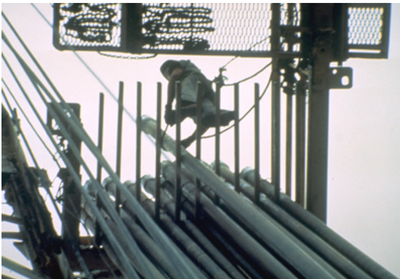
Figure 6. The derrick employee, standing on the fingerboards in this view, moved pipe between the pipe racks and the wellbore during trips in and out of the hole. This job was physically demanding and required wearing a safety harness when up in the derrick. Today the operation of drill pipes has been automatised. Photo: Schlumberger Limited.
