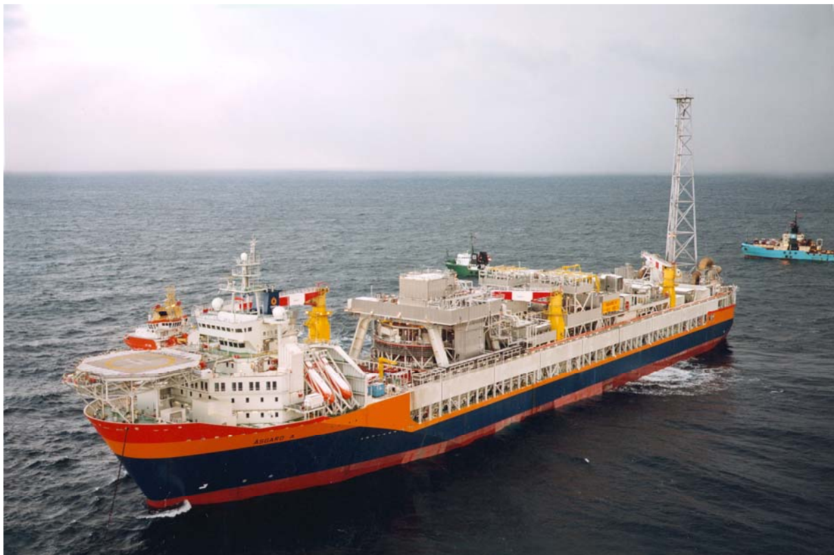
Figure 2. Norwegian oil companies have preferred building more easily removable production ships in the past decade due to smaller oil and gas fields and for environmental reasons. This picture shows an oil and condensate processing production and storage vessel: Åsgard A. Photo: Statoil.
