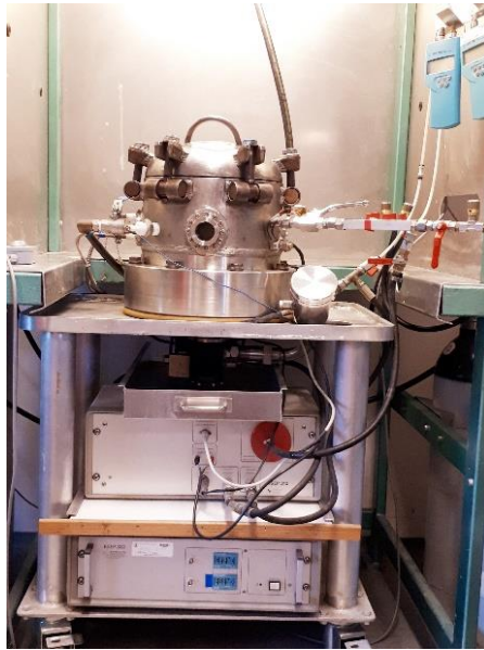
Figure 3.2: The 20-litre explosion vessel and associated systems
