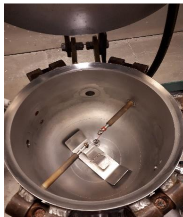
Figure 3.4: A 1 kJ chemical igniter (left) and the igniter fixed in the centre of the vessel (right).
