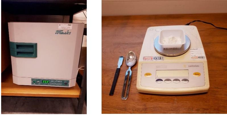
Figure 3.5: The oven (left) and scale (right) used for drying and weighing dust samples.
