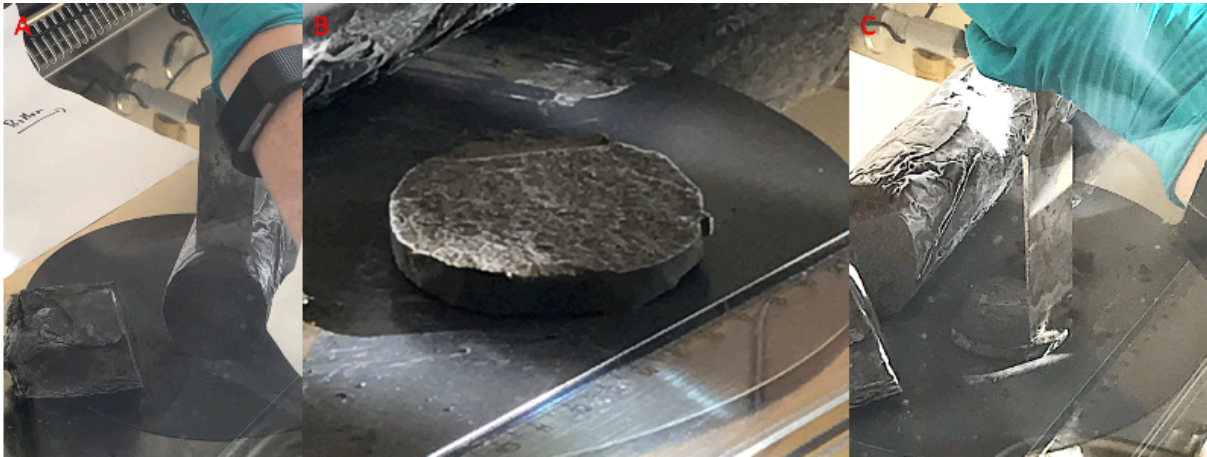
Figure 3: Process of subsampling the 2016 fragments. A. Samples cut by sterile chisel. B. ~1 cm thick fragment. C. Cutting of the outer part with sterile chisel.
