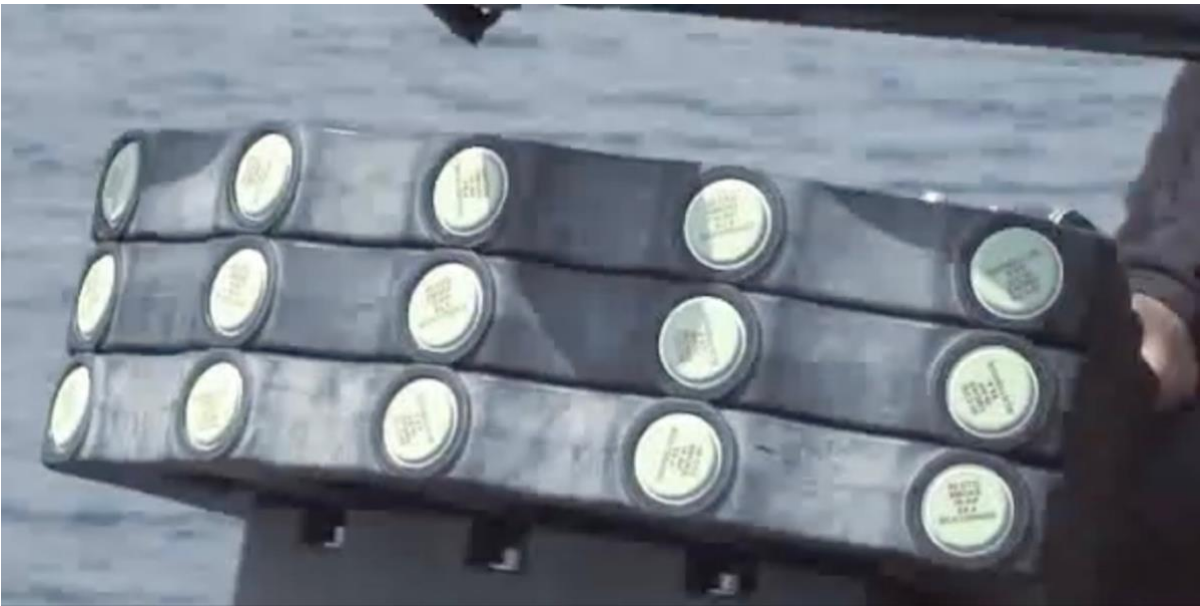
Bilde 3: Rosy N- Rapid Obscuring system (Rheinmetall)
