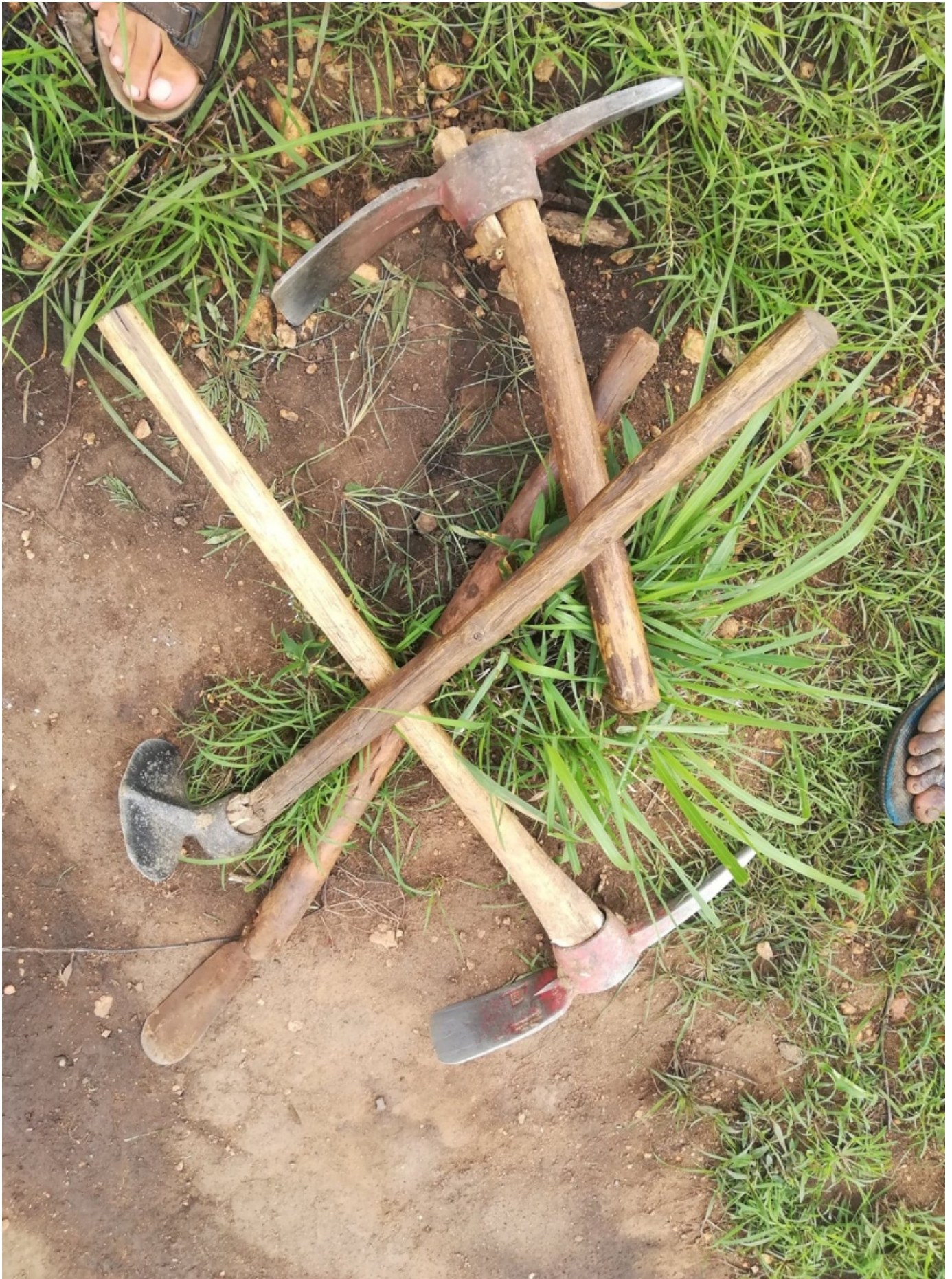
Picture 2: Tools used for digging latrines and graves get quickly worn down because of the rocky soil. Photo: Mikko Virtanen
