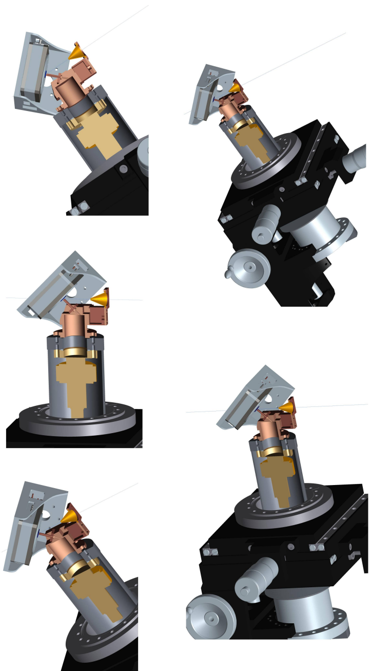
Figure 6.54: Sketches of the reflection detector mounting from different view directions and with different magnifications with the reflection detector and the extension tube shown in a half section sketch for better illustration. The stage is mounted from outside on the sample chamber (see section 6.3.3).
