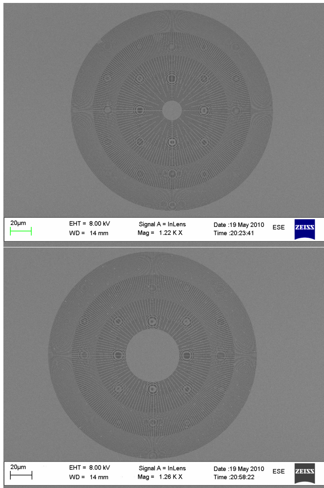
Figure 4.4: Scanning-electron micrographs showing the two different zone plate types utilized in the NEMI setup representing the difference in the middle stop diameter; top: outer diameter d_{ZP} = 192\ \mu\text{m} zone plate with a middle stop diameter of d_{MS} = 20\ \mu\text{m} (support chip 8, membrane 2); bottom: d_{ZP} = 192\ \mu\text{m} zone plate with a middle stop diameter of d_{MS} = 50\ \mu\text{m} (support chip 8, membrane 6). (again the in a circular wave form shaped patterns overlying both micrographs are imaging artifacts)
