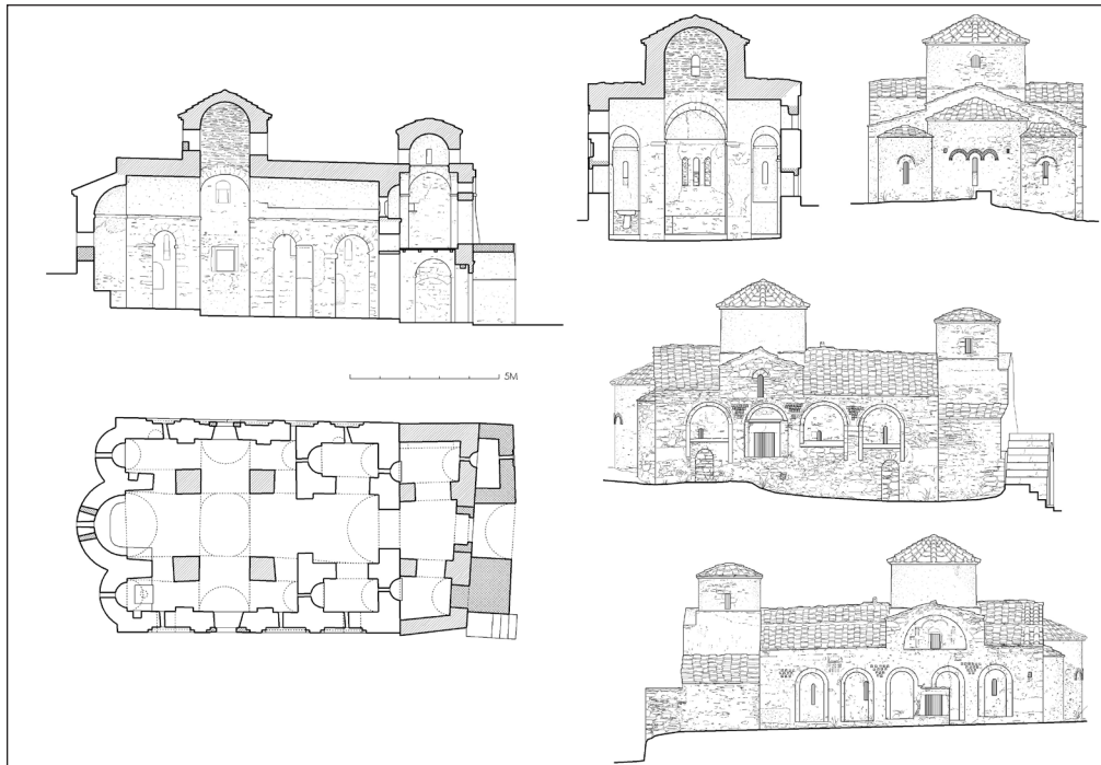
Figure 33. Agioi Apostoloi at Metochi. Plan, sections, north, south and east elevations.
