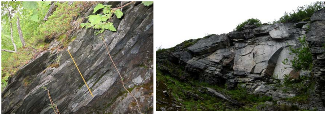
Figure 10. Rock outcrops. Left: dense jointing along the foliation. Right: dense jointing along the foliation with more massive rock above.
