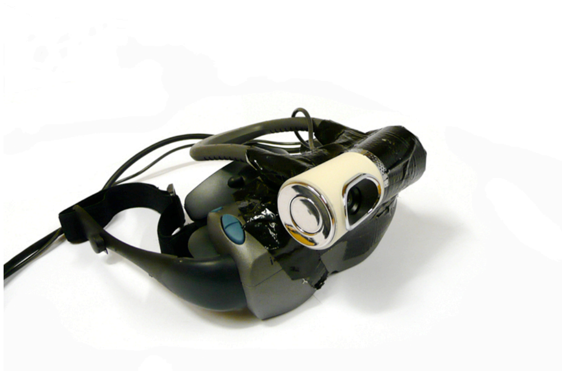
Figure 8: The HMD mounted with the web camera using pipe tape.
