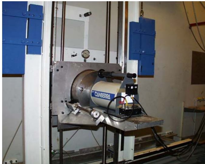
Figure 3.1 Vertical rig for 2-D in-situ saturation measurement.
