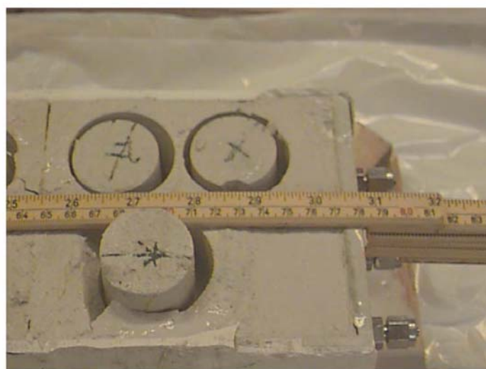
Figure 3.4 Drilling of core plugs from blocks to verify wettability conditions.
