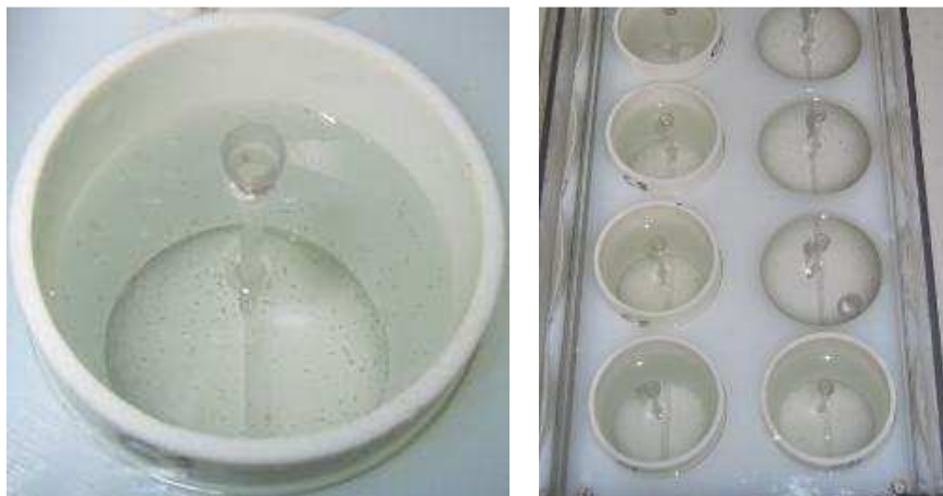
Figure III. Lice incubators with newly hatched L. salmonis nauplii larvae. Water is supplied through the nipple in centre.
