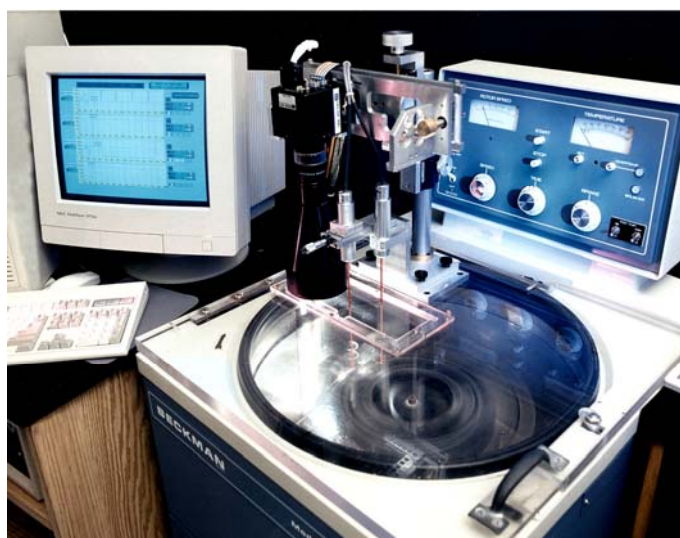
Figure A1. Automated centrifuge system with a standard centrifuge, a high spatial resolution camera for production measurements and a computer for running the software and storing data. Each production measurement is fully automated, reducing the need to supervise the experiment and limits biased experimental readings.
