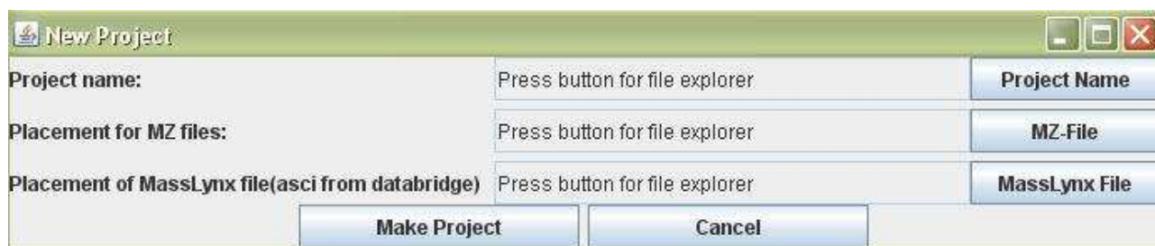
Figure 5.3: Shows the window for a new project and the information that needs to be filled in to create a new project.
