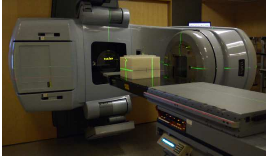
Figure 6.4: Experimental setup for the in-phantom measurements at Haukeland University Hospital. The isocenter is placed at 8.57 cm depth in the phantom.
