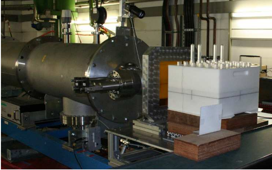
Figure 6.5: Experimental setup in cave A at GSI. The beam pipe to the left is followed by an ionization chamber and the plastic phantom.
