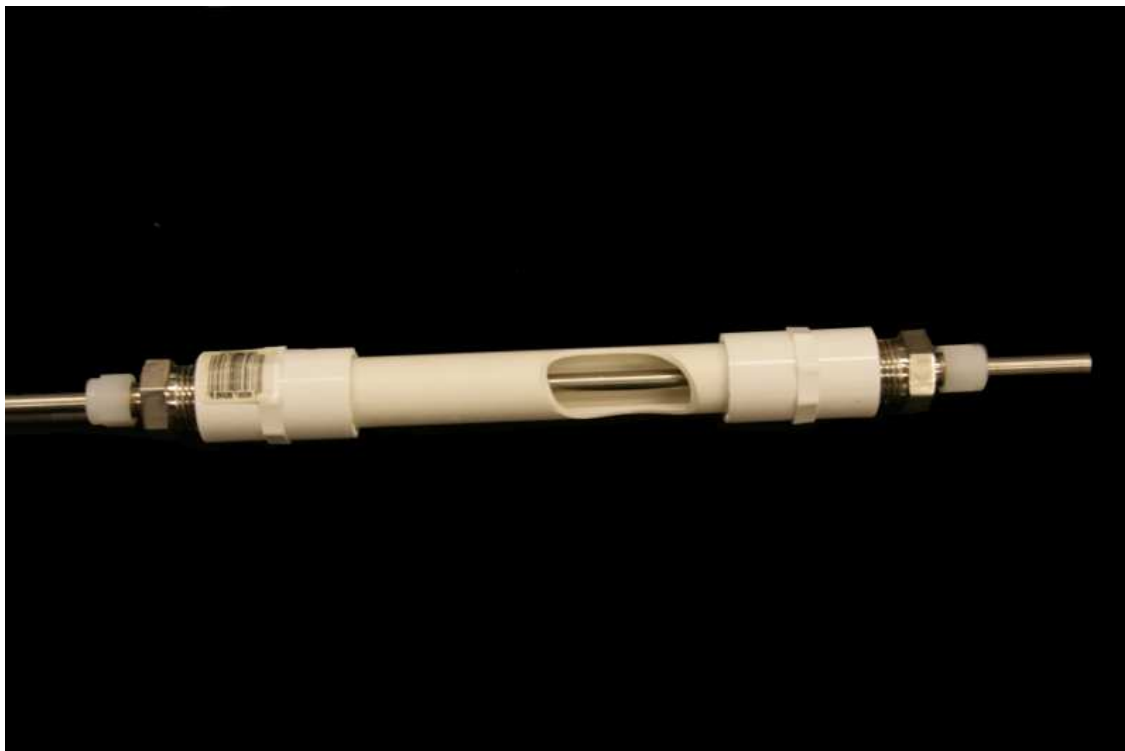
Appendix B3 – Illustration of tube in tube where Fluorinert is circulating in the inner tube, and antifreeze is circulating in the outer PVC tube and maintaining low temperature of Fluorinert.
