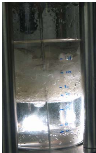
Figure 3.5: Dissociation of propane hydrate plug by two-side depressurisation in the laboratory (photo by Kristin Erstad, Department of Chemistry, University of Bergen, 2006).
