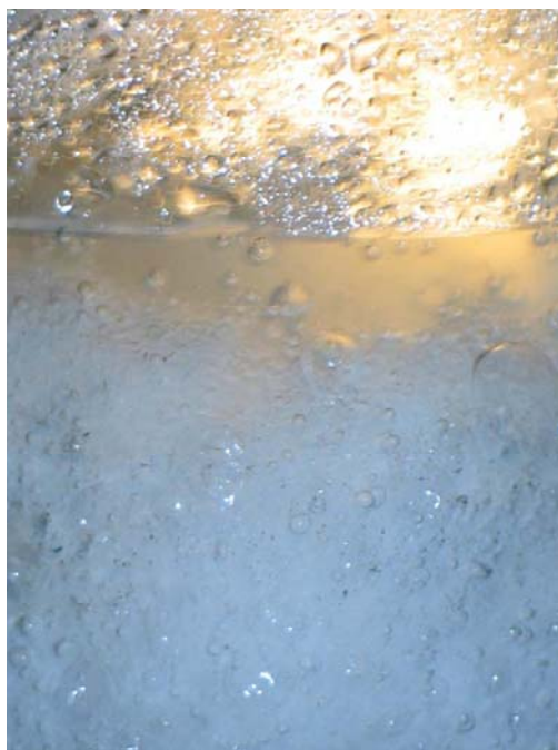
Figure 3.1: Decomposing propane hydrates (photo by Kristin Erstad, Department of Chemistry, University of Bergen, 2006).
