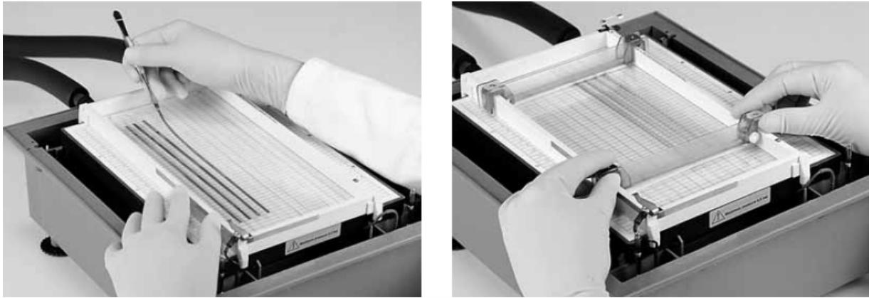
**Figure 2-2: Positioning of the IPG–strips in the Drystrip aligner and connection of the electrodes (GEHealthcare 2004).**
