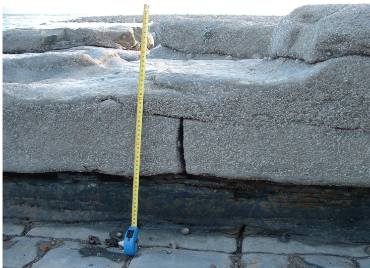
Figure 4.2: A hydrofracture has joined with a weak horizontal contact resulting in a T-shaped fracture. The steel tape has a length of 50 cm.
