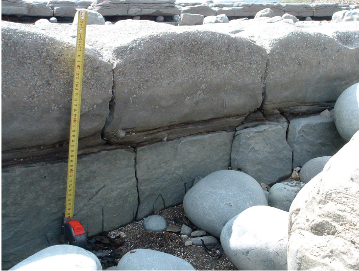
Figure 4.1: Hydrofractures propagating through a mechanically layered sedimentary rock of alternating stiff limestone and soft shale layers, near to Llantwit Major, South Wales. Due to the low or zero tensile strength of the soft shale layer, the hydrofractures must follow shear fractures to continue their propagation as they enter the shale.
