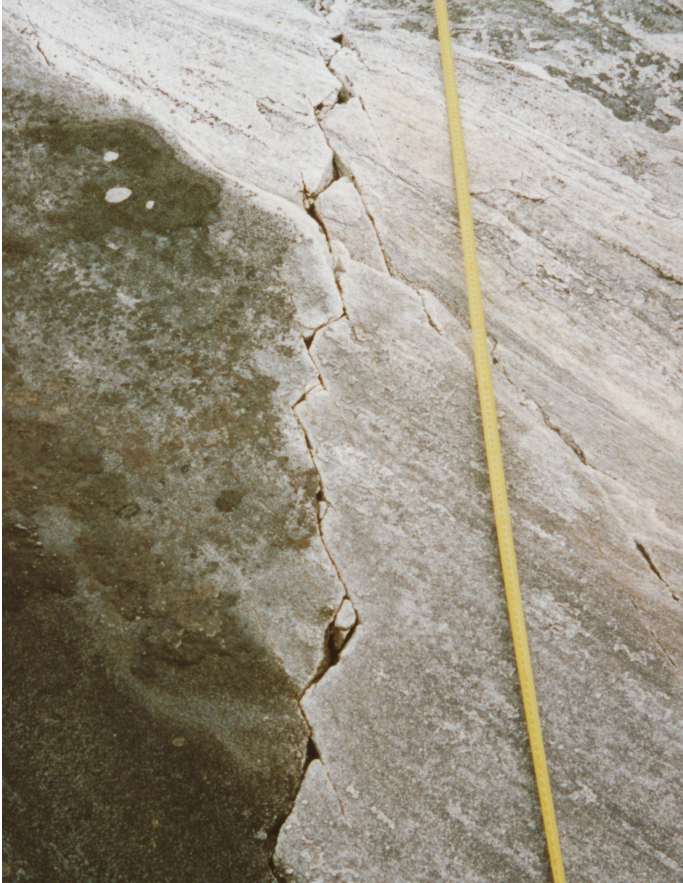
Figure 6.2: Extension fractures linked up through transverse shear fractures in Øygarden. View is south-southwest; the length of the steel tape is 1.5 m.
