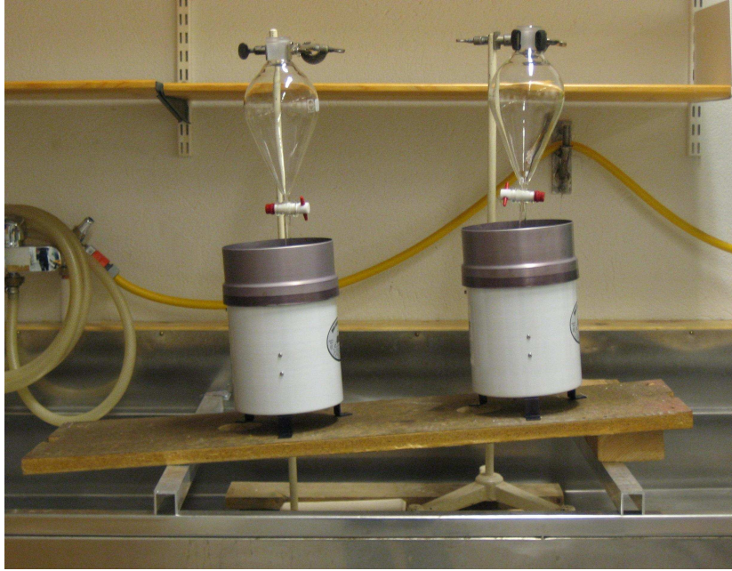
Figure 9: Laboratory setup for the test of non-level mounting on the sampling efficiency of HOBO rain gauges.
