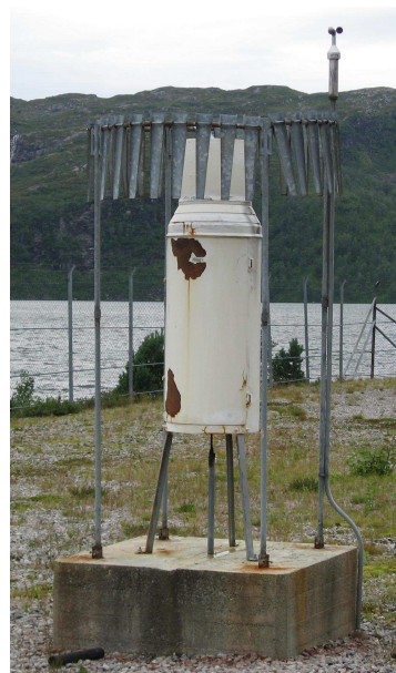
Figure 8: SIAP rain gauge situated at the power station area at Stordal.
