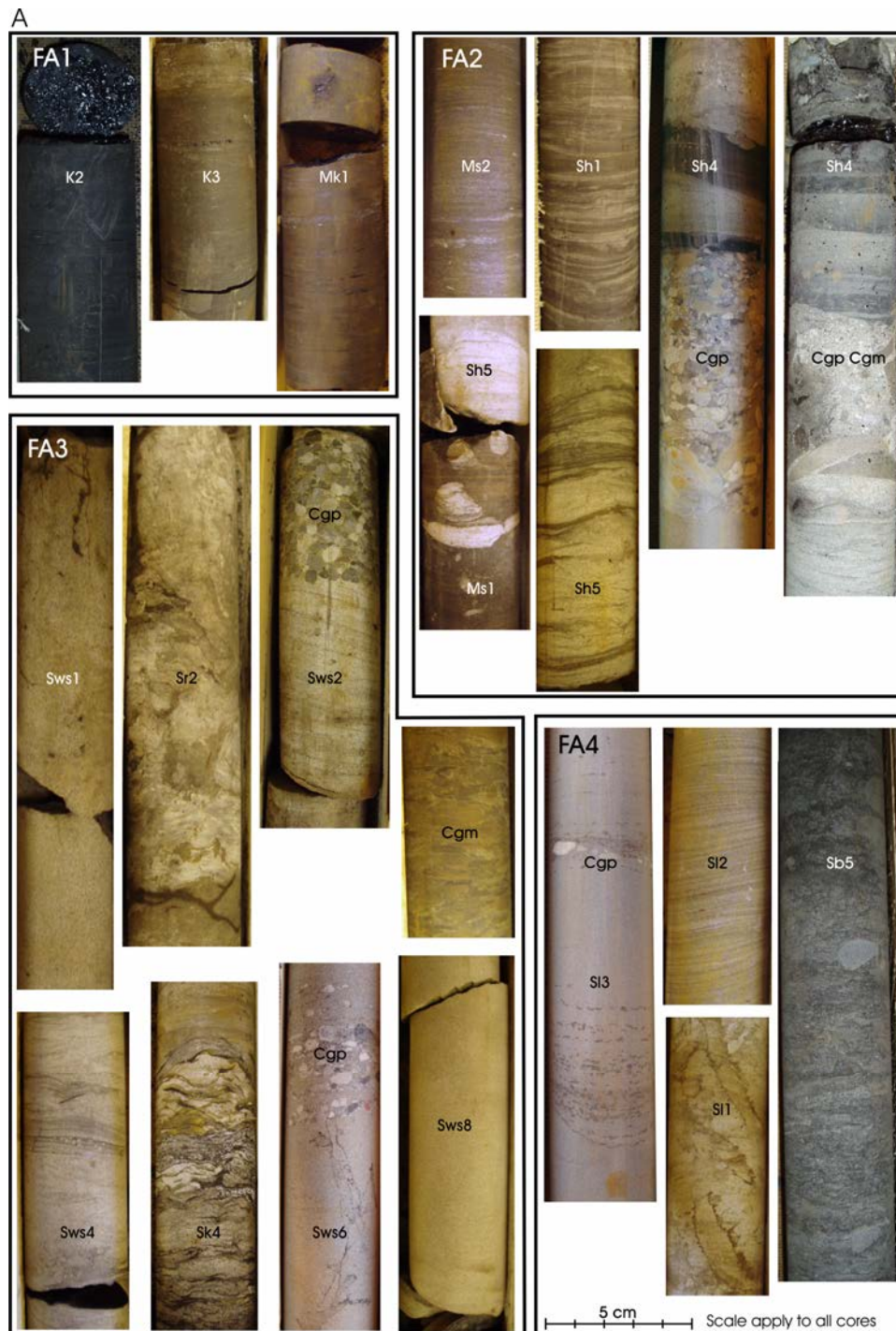
Fig. 4 (A) Core photographs representing the facies recognised in the study area, grouped by facies associations. FA1 vegetated subaerial to marginal marine; variations of muddy coal and carbonaceous mudstone. All coal is sampled at the drill site for geochemical analysis. FA2 back barrier tidally influenced lagoon; variations of tidal deposits and different conglomerate. Notice sandfilled centimetre scale burrows. FA3 barrier bars; foreshore/upper shoreface well sorted sandstone, different related conglomerates, paleosol represented by Sr2 rooted sandstone, and Sk4 organic-rich sandstone wash-over/flooding surface. FA4 shoreface and offshore transition; range of sandstone from storm deposited well sorted shoreface to muddy bioturbated lower shoreface with large scale Ophiomorpha .
