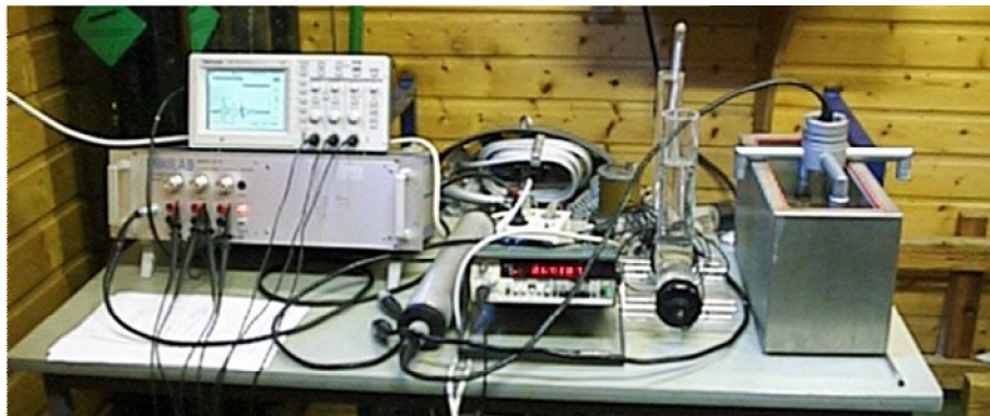
Figure 2.5: a) Velocimeter schematic set-up (redrawn from Kristensen, 1983, and Køgeler et al., 1987). b) The Espegrand 1998 sound speed measurement bench-work .
