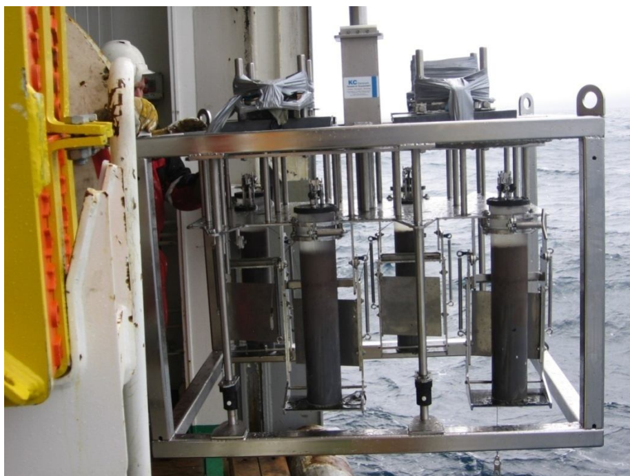
Fig. 3.2: Picture of the GS06-144-09 MC A-D core coming up after a successful multi-core operation. Photo by Ulysses S. Ninnemann.
