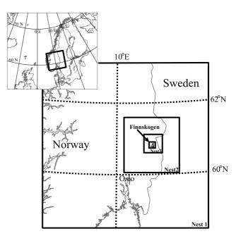
**Figure 1.** Nesting of MM5 domains. All domains are 40  $\times$  40 grid points with the resolution 13.5 km  $\leftrightarrow$  4.5 km  $\leftrightarrow$  1.5 km  $\leftrightarrow$  0.5 km (Nest1...Nest4). The upper left figure shows the position of Nest 1 on an European scale.
