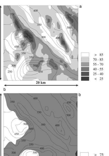
**Figure 4.** (a) Calculated net shortwave radiation (SW) at the surface,  $Wm^{-2}$ , in the modified-run at 16 UTC 20 September 1994. Shaded areas show minima of SW, white areas maximum. Isolines are height of topography. The model grid distance is 500 meters. (b) The reference run.
