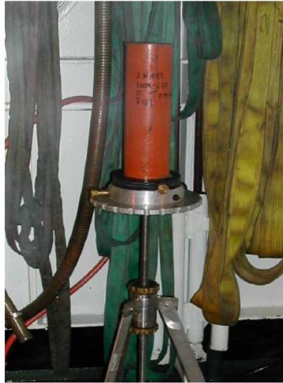
Figure 2.5: Corer cutting device; photo: Hilde Elise Haldal.
