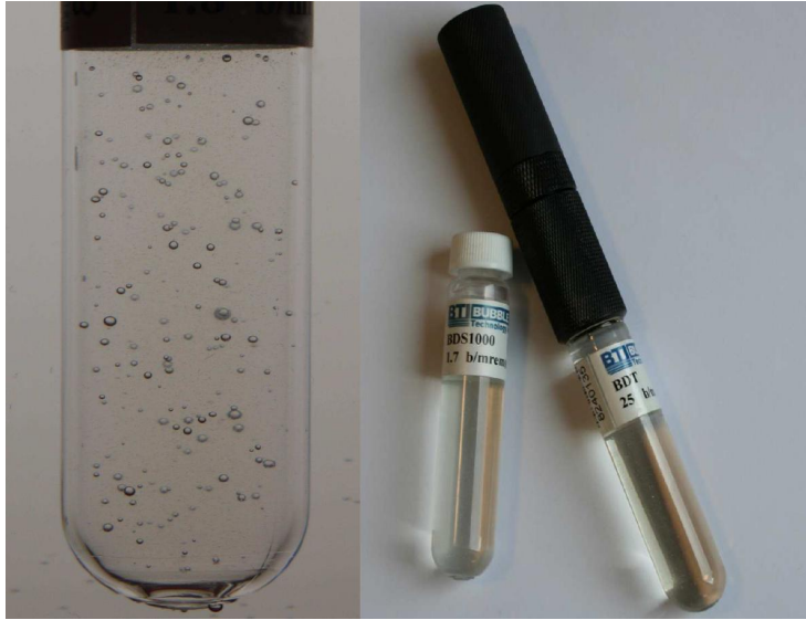
Figure 5.1: Bubble detectors. Left image shows a bubble detector after exposure to neutrons. Right image shows two unexposed types of bubble detectors.
