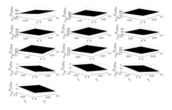
**Figure 5** Real part of the independent effective stiffness constants as a function of fracture densities ( $\varepsilon_1$ ,  $\varepsilon_2$ ) for two fracture sets for a frequency of 40 Hz. The azimuthal orientations for fracture set 1 and 2 are equal to 35° and 108°. The fracture radius of both the aligned mesoscopic fracture sets and matrix permeability was set to 0.1 m and 100 mD.
