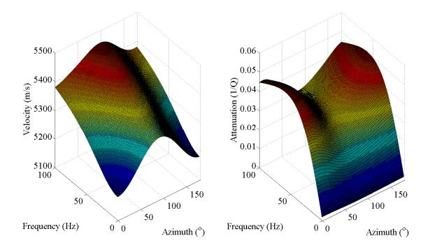
**Figure 11** Seismic velocity and attenuation data as a function of seismic frequency and azimuth for a fixed polar angle of incidence (40°). The azimuthal fracture orientations ( $\psi_1$  and  $\psi_2$ ) and fracture densities ( $\varepsilon_1$  and  $\varepsilon_2$ ) of the two mesoscopic fracture sets are equal to (35°, 108°) and (0.03, 0.05) in this particular example.
