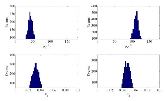
**Figure 13** Samples of the marginal posterior PDF's for azimuthal fracture orientations ( $\psi_1$  and  $\psi_2$ ) and fracture densities ( $\varepsilon_1$  and  $\varepsilon_2$ ) using measurements of both seismic velocity and attenuation anisotropy data corresponding to different seismic frequencies and azimuths. The standard deviation of measured seismic velocity and attenuation data was set to 25%.
