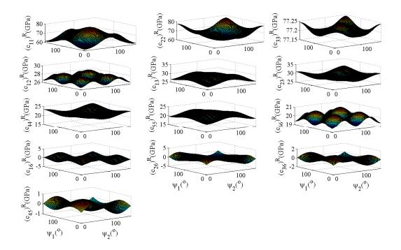
**Figure 3** Real part of the independent effective stiffness constants as a function of azimuthal fracture orientations ( $\psi_1$ ,  $\psi_2$ ) for two fracture sets for a frequency of 40 Hz. The fracture densities for the fracture set 1 and 2 are equal to 0.03 and 0.05. The fracture radius of both the aligned mesoscopic fracture sets and matrix permeability was set to 0.1 m and 100 mD.
