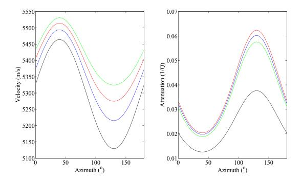
**Figure 7** Azimuthal variation of P-wave velocity (left) and attenuation (right) for different seismic frequencies and a fixed polar angle of incidence  $(40^{\circ})$  in a medium with one fracture set. The azimuthal orientation of the mesoscopic fracture is  $40^{\circ}$ . Black lines: 20 Hz, blue lines: 45 Hz, red lines: 65 Hz and green lines: 90 Hz.
