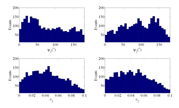
**Figure 12** Samples of the marginal posterior PDF's for azimuthal fracture orientations ( $\psi_1$  and  $\psi_2$ ) and fracture densities ( $\varepsilon_1$  and  $\varepsilon_2$ ) using only measurements of seismic velocity anisotropy data corresponding to different seismic frequencies and azimuths. The standard deviation of measured seismic velocity data was set to 25%.
