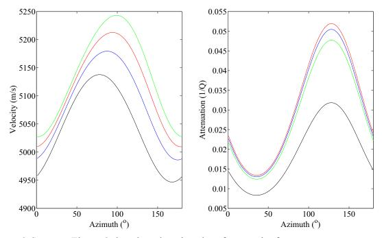
**Figure 9** Same as Figure 9, but the relaxation time for one the fracture set was set equal to micro-porosity. Black lines: 20 Hz, blue lines: 45 Hz, red lines: 65 Hz and green lines: 90 Hz.
