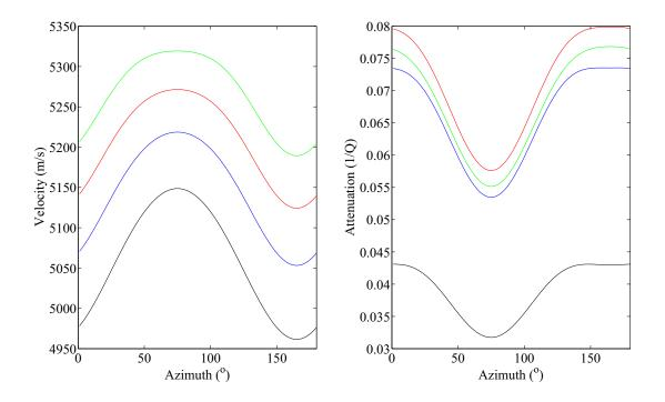
**Figure 8** Azimuthal variation of P-wave velocity (left) and attenuation (right) for different seismic frequencies and a fixed polar angle of incidence  $(40^{\circ})$  in a medium with two fracture sets. The azimuthal orientations of the two mesoscopic fracture sets are  $40^{\circ}$  and  $110^{\circ}$ . Black lines: 20 Hz, blue lines: 45 Hz, red lines: 65 Hz and green lines: 90 Hz.
