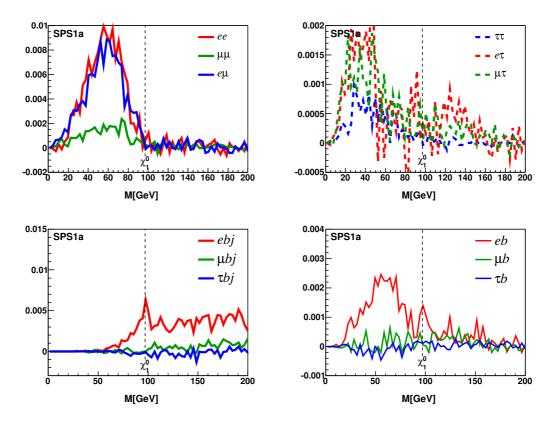
Figure 15. Mix of operators: Invariant mass distributions for  $\lambda_{121} = 10^{-5}$  and  $\lambda'_{123} = 10^{-4}$  at SPS1a. Upper panels: di-lepton invariant mass distributions. Lower left panel shows  $\ell b_{\rm jet} j$  and lower right shows  $\ell b_{\rm jet}$ .
